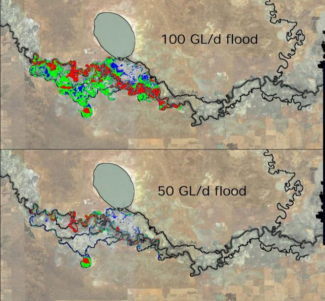
Aquaterra developed specific recharge rates (mm/day) to apply to AEM salinity index product values/classes (provided by SKM & Ray Evans, see previous slide), and to inundation extents from hydrodynamic model (WaterTech)
