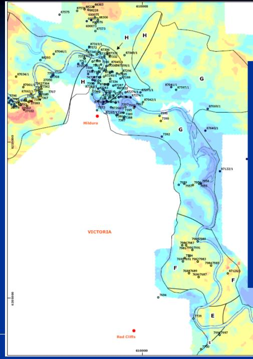
**AEM Survey (colour** flood) matches TDS salinity at bore points. EM2 model uses distributed AEM on each grid cell for near-river salinity for salt load calc, instead of zoned/averaged TDS from bore points.
