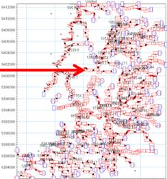
Geological model constructed using scripts to transform GIS rasters directly to MIKE SHE .dfs2 files
